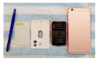
2 Align the alignment paper card at the lower edge of the camera lens and in the central part of the phone.
